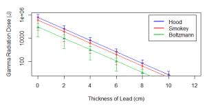
Figure 2: Gamma radiation dose Indiana receives with varying thickness of lead.
