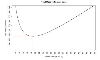
Figure 1: A plot of the relationship between the total mass,  $M_t$ , and mass of the reactor,  $M_n$ . The minimum total mass occurs at the turning point, marked by the red circle and lines.
