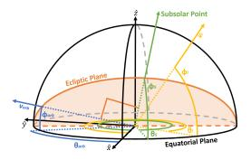
Figure 1: A diagram showing the system on the northern hemisphere, where blue components are for  $v_{orb}$ , orange components are in the ecliptic plane, green components are for the subsolar point, yellow components are for  $v_l$  and black components are the Earth outline.
