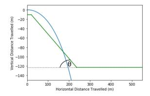
Figure 2: A more realistic trajectory of the rocket powered MINI - blue line - by using a velocity of  $45 \text{ ms}^{-1}$ .
