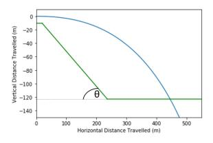
Figure 1: A plot showing the trajectory of the rocket powered MINI - blue line - using a final velocity of 110 ms<sup>-1</sup>. The green line represents the hill, which we estimate starts 10m below the jump.  $\theta$  represents the angle of the slope, 27 degrees.
