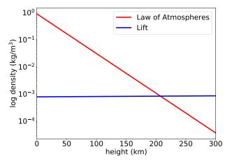
Figure 1: A plot of the particle density required for a plane to reach maximum lift (blue), and that of a hypothetical Mars atmosphere with increasing height (red). The two lines intersect at  $\sim 210$  km.
