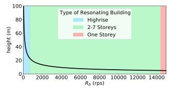
Figure 1: The relationship between the firing rate and the height of the building that will resonate with the corresponding earthquake (Eq. 6).
