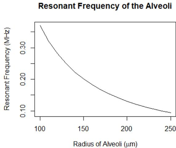
Figure 1: Shows how the resonant frequency changes with the radius of the alveoli. As the alveoli expands the resonant frequency decreases from 0.3701 MHz to a value of 0.0936 MHz.
