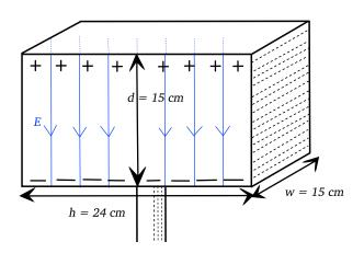
Figure 1: Mjolnir shown with its measurements, as well as the positive and negative plates, which form the capacitor. The electric field, E, is shown in blue.
