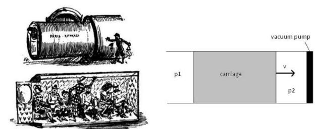
Figure 1: Left, Robida's original sketch. Right, diagram of proposed pneumatic tube train.
