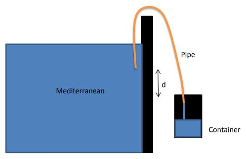
Fig 1 shows a siphon system where d is the difference between the vertical displacements of both ends of the Pipe.
