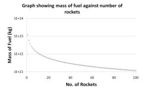
Fig.1 Graph showing the mass of fuel against the number of rockets required to perform the first half of the Hohmann transfer.
