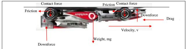
**Figure 1**: A simple force diagram of a Formula one car that is driving on the ceiling, here the downforce must be greater than the weight of the car in order for it to experience any traction from the ceiling. (Image credit adapted from: www.blogspot.com) [1]
