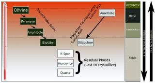
Figure 1: Bowen's Reaction Series showing the lower temperatures at which quartz crystallizes [7].
