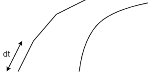
Figure 1: Diagram illustrating why the choice of time step is important. The left is our approximation and the right is the true curve. If we had a smaller time step, so more lines, it would fit the curve better.
