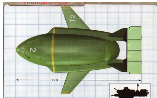
Figure 1: A diagram showing the dimensions of Thunderbird 2 each square is 23 \times 23\text{ft} [2].
