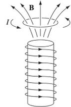
Figure 1: Example solenoid with a magnetic field moving in the positive  $z$  direction [2]
