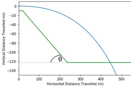
Figure 1: A plot showing the trajectory of the rocket powered MINI - blue line - using a final velocity of  $110 \text{ ms}^{-1}$ . The green line represents the hill, which we estimate starts 10m below the jump.  $\theta$  represents the angle of the slope, 27 degrees.
