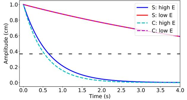
Figure 1: The amplitude of the high E (blue) and low E (red) strings as a function of time, for a solid (solid) and chambered (dashed) guitar. The black dashed line is at  $e^{-1}$ , where  $A = A(2\tau)$ .
