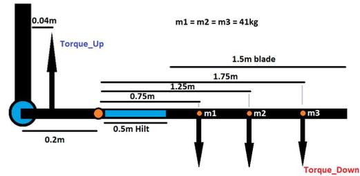
Figure 1: Model used to calculate the exerted force onto the sword, from the bicep.(Equation 4). The pivot point (elbow) being the centre of the blue circle on the left.
