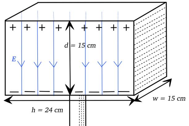
Figure 1: Mjolnir shown with its measurements, as well as the positive and negative plates, which form the capacitor. The electric field,  $E$ , is shown in blue.
