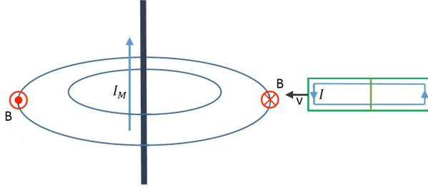
Figure 1: Magneto is idealised as an infinitely long straight wire. A projectile with velocity  $v$  approaches him and, as a consequence, an anticlockwise Eddy current is generated inside the moving object.
