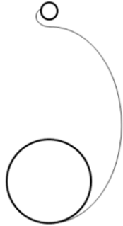
Figure 1: The most efficient orbit to reach the Moon.
