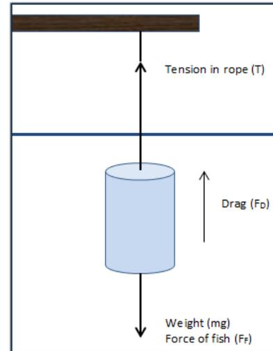
Figure 1: Diagram of force acting on net
