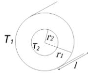
**Figure 1:** Schematic of the superconducting wire, of length,  $l$ , with an insulating layer with an inner radius  $r_2$ , at a temperature  $T_2$ , and an outer radius  $r_1$ , at an ambient temperature  $T_1$ .
