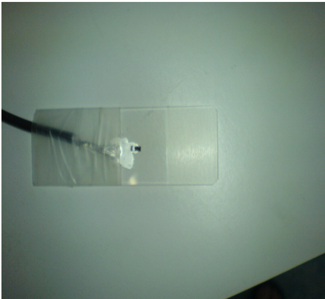
Figure 4b: An image of the sample on a glass slide with a wire that leads to the multimeter and the silver solution used to establish an electrical connection between the two.
