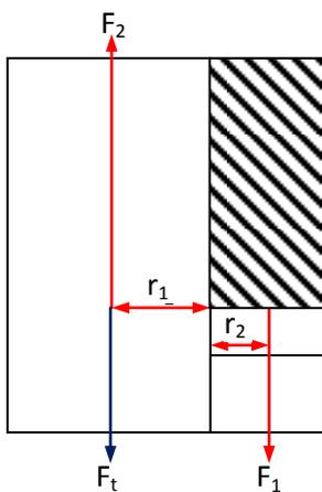
Figure 1: Side view of a tree after 50,000 punches. The hatching shows the section that would be acting downwards, pulling on the tree.  $F_1$  is the force due to gravity on the overhang and  $F_2$  is the force this exerts on the still attached section of tree.  $F_t$  is the force holding the tree together.  $r_1$  and  $r_2$  are the distance that the centre of each force is from the pivot point.
