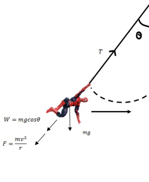
Figure 2: Calculating tension in spider web
