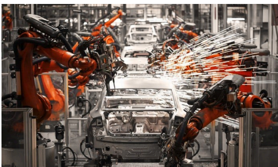
Figure 2 – Image of a car assembly line with automated machine arms being used to construct the frame [14].
