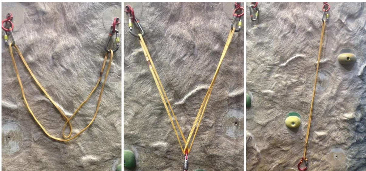
Figure 1 – A series of photos showing the Magic X anchor before clipping (left), fully constructed and clipped (middle), and it after the failure of one anchor point (right). The anchor is constructed by clipping two locking carabiners into two anchor points (two bolts in this case), attaching a sling to these, making a twist in one of the two strands created by this, and finally clipping another locking carabiner through the twisted and un-twisted strand. This third carabiner (red) is where the climber would attach themselves to. Professional instruction should be sought prior to using this technique on real rock.
