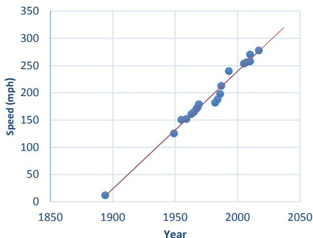
Figure 1 – Trend of production car top speed
