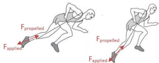
Figure 1 –  $F_{applied}$  and  $F_{propelled}$  are equal and opposite forces [7]. Horizontal starting positions (left) direct greater portions of  $F_{propelled}$  forward than vertical starting positions (right) [6, 7].
